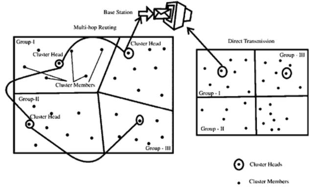
Fig 4.1: LEACH Operation Showing Set-up, Steady State Phases using Multi-hop, also Showing Direct Transmission
