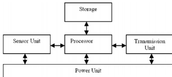
Fig 1.1: Logical Diagram of a Wireless Sensor Networks
