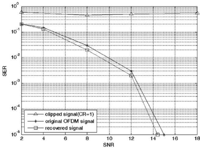
Fig. SER Performance of Clipped and Recovered OFDM Signals
