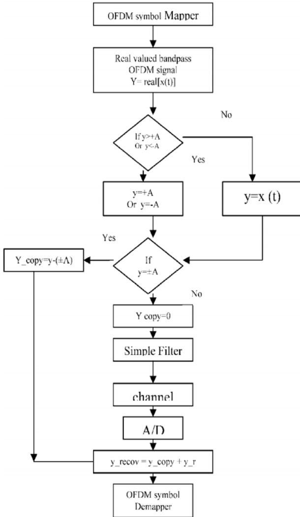
Fig. 3: The Proposed Method to Recover the Clipped OFDM Signal
