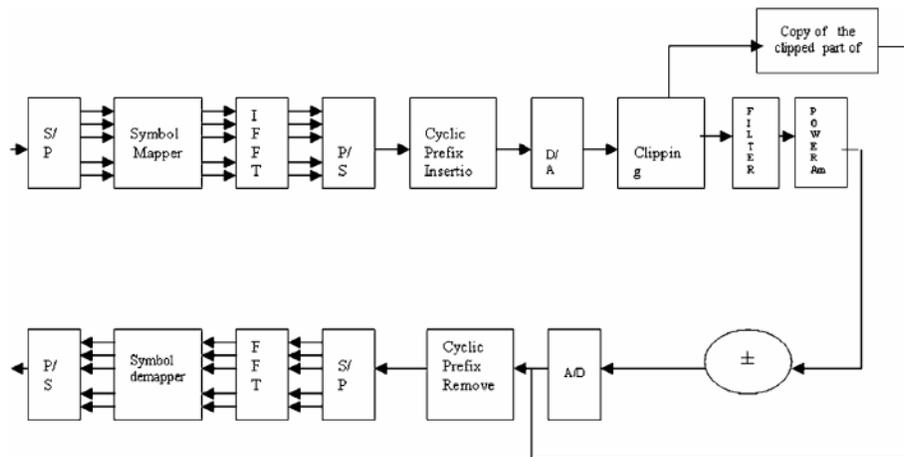
Fig. 1: OFDM System Block Diagram and the Proposed Solution
