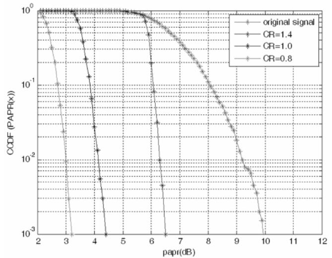
Fig: CCDF of PAPR for Normal and Clipped OFDM Signal at Different CR with 16-QAM
