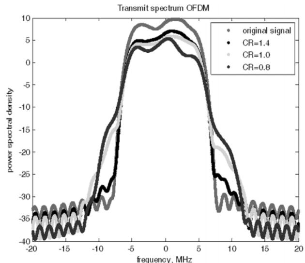
Fig: Spectrum of Clipped OFDM Signal
