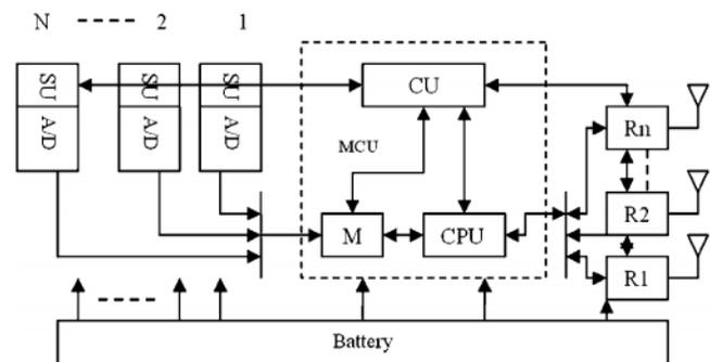
Fig. 1.1: Architecture of Sensor Nodes [3]
