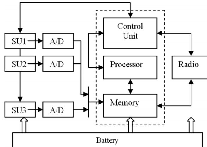
Fig.1.5: Sensor Node Architecture (Fine-Grain Scheduling within a Sensor Node)
