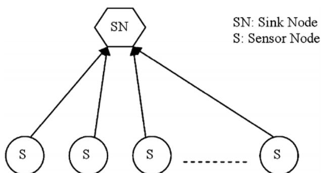
Fig. 1.2: Single-hop Multi-source Sensor Network (SHMS)
