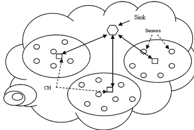
Fig.1.4: System Model (Coarse-Grain Scheduling in a Sensor Group)
