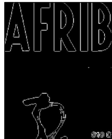
Fig.3: Fuzzy Edge Filter at Specified Threshold
