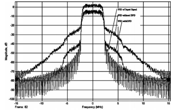
Figure 7: Performance of Pre-distorter in Suppressing Spectral Regrowth
