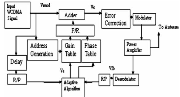
Figure 5: Block Diagram of Adaptive Digital Pre-distorter
