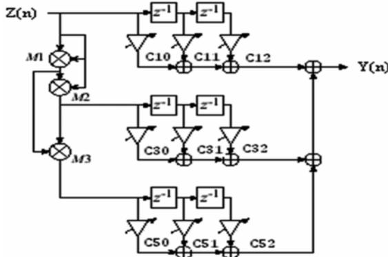
Figure 2: Direct form Realization of the Modified Memory Polynomial
