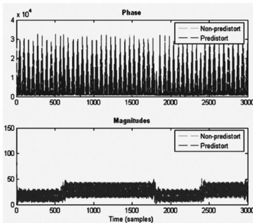
Figure 6: Magnitude and Phase Errors with and Without Pre-distortion
