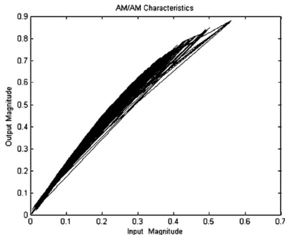
Figure 3: AM-AM Characteristics of the PA Model
