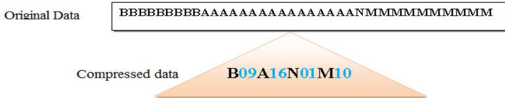
**Fig 3: Run-length encoding compressed data.**
