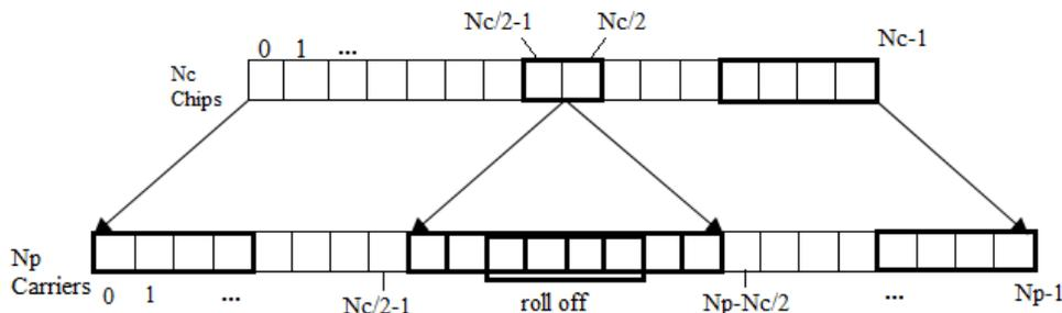
Figure 3: Mapping of chips on the carriers [7]
