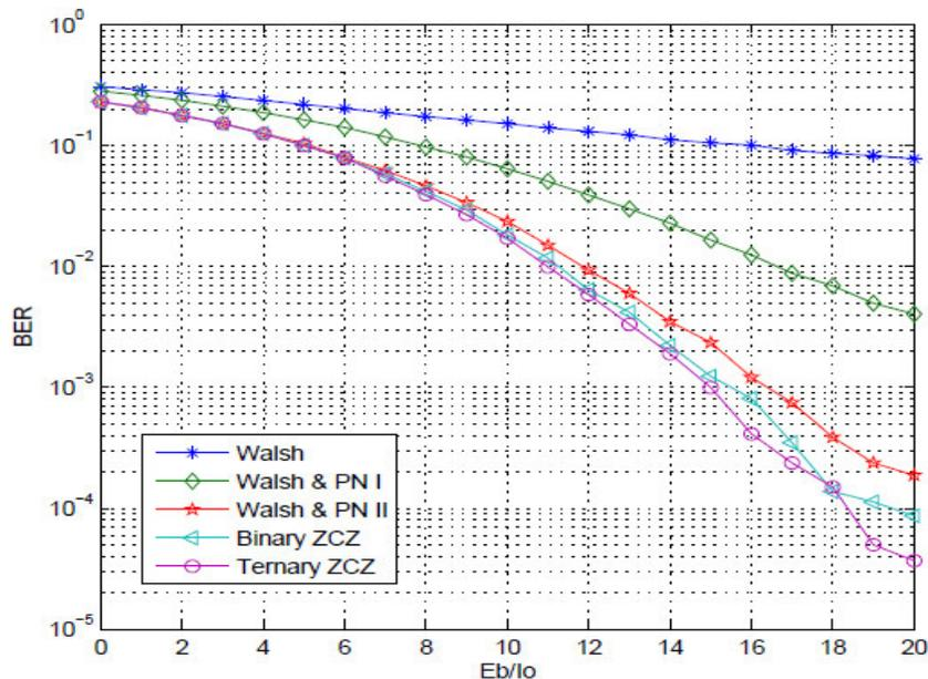
Figure 5: Bit error rate versus signal to noise ratio over Multipath Rayleigh fading channel [8]
