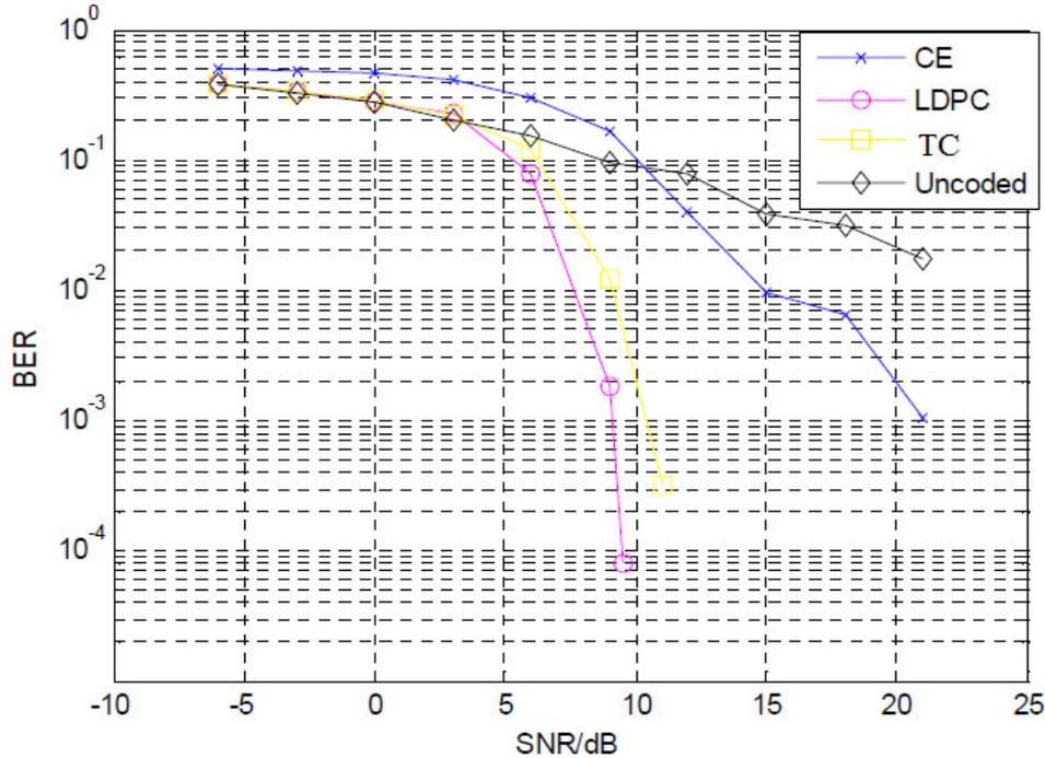
Figure 6: Coded Multi Carrier-Code Division Multiple Access performance for Rayleigh Fading channel [15]
