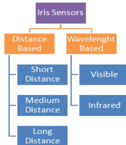
Fig. 2 Classification of various Iris sensors.
