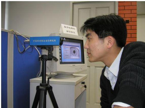
Fig 4. Example of medium distance based iris camera.
