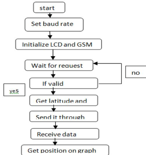
Figure 2. Flow chart of GPS tracking system
