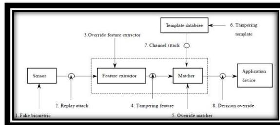
Fig 4 attack point on biometric system
