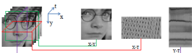
Fig. 2 The textures in XY, XT and YT planes.
