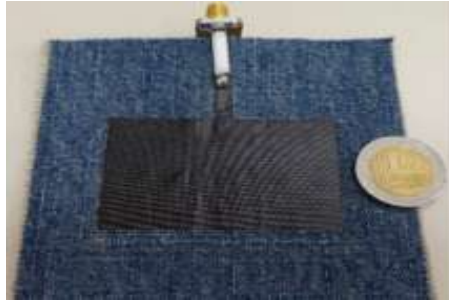
Fig 4 Wearable antenna using jeans substrate
