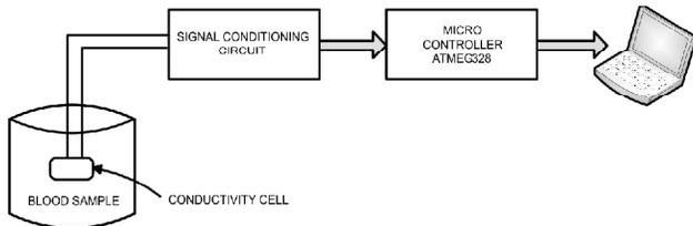
**Figure 1: Block Diagram Human Blood Conductivity System**
