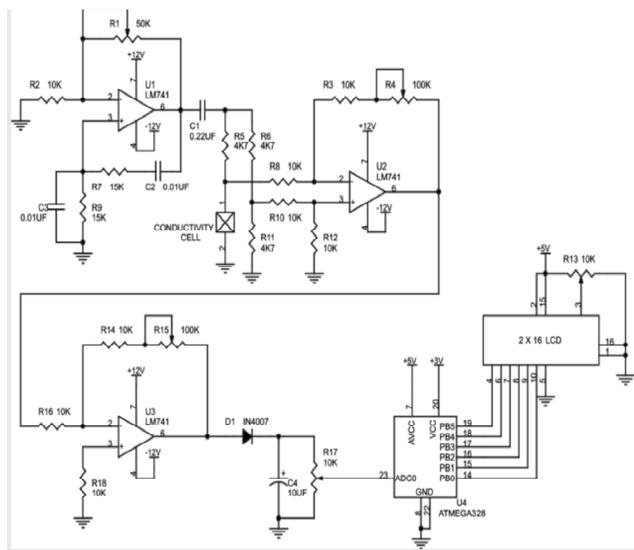
**Figure 2: Schematic Diagram of Microcontroller based Human Blood Conductivity Measurement System**
