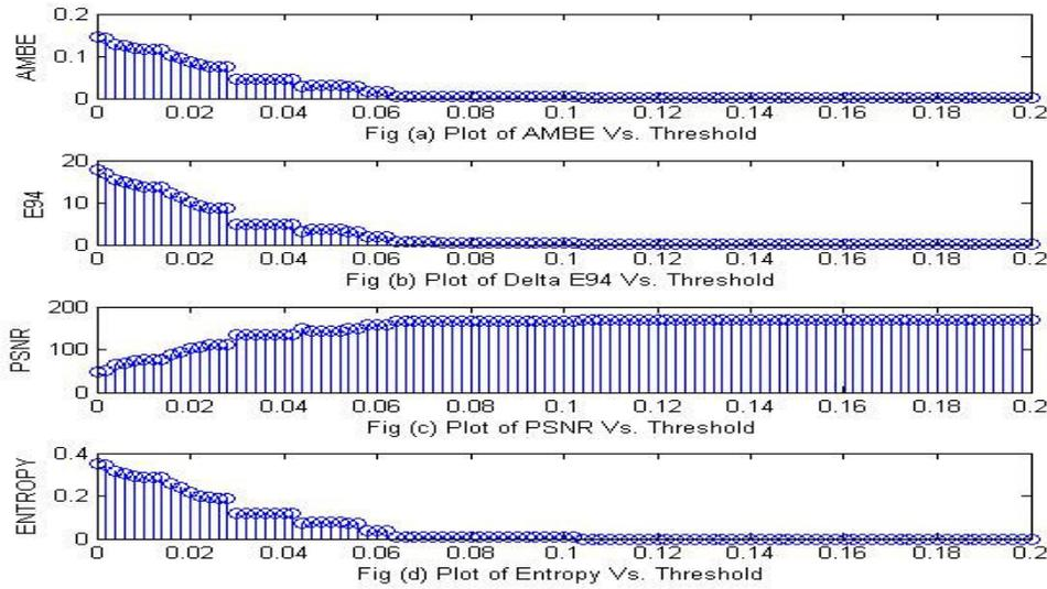
Fig. 1 Plots of video contrast enhancement quality metrics (a) AMBE versus Threshold (b)  $\Delta E94$  versus threshold (c) PSNR versus threshold (d) Entropy versus threshold, study of the Temporal Based (TB) method as applied for video-contrast enhancement by varying  $T_n$
