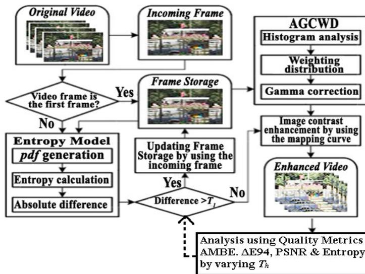
Fig. 1 Flowchart of the Temporal Based (TB) method as applied for video-contrast enhancement by varying  $T_h$
