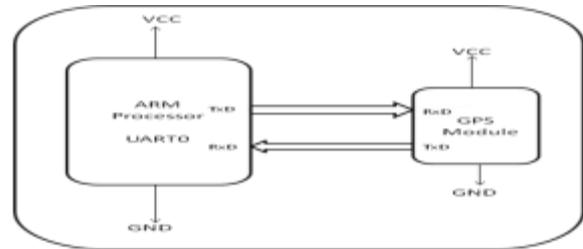
Figure 10. Interfacing of GPS with ARM UART0
