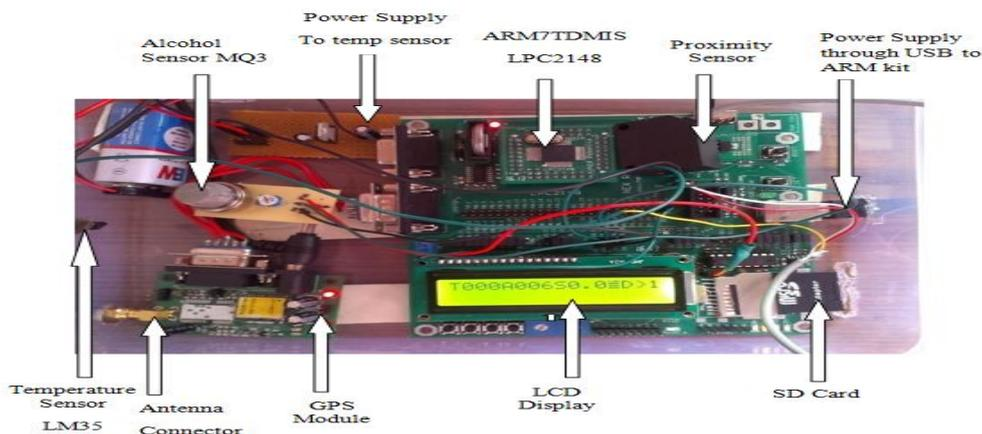
Figure 2. Implementation of Event Data Recorder (First System)
