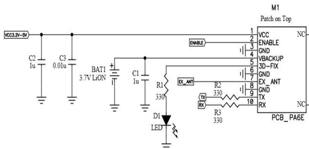
Figure 9. UART interface with ARM
