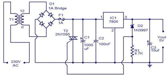
Fig. 6. A 5V regulated power supply.
