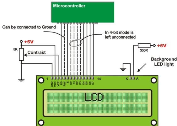
Fig. 5. Interfacing Diagram of LCD with Microcontroller.
