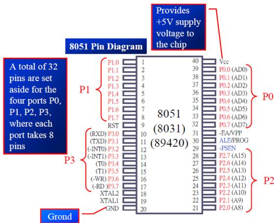
Fig. 2. Pin Diagram of the 8051 Microcontroller.
