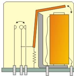
Fig. 4. Internal Construction of a Relay.
