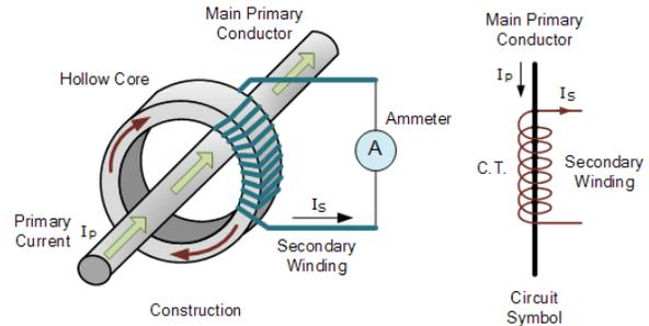
Fig. 3. Working Principle of a Current Transformer.
