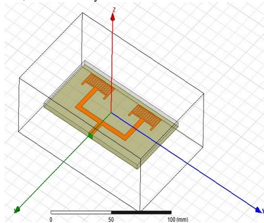
Figure3. Design of 2x1 Slotted microstrip patch antenna
