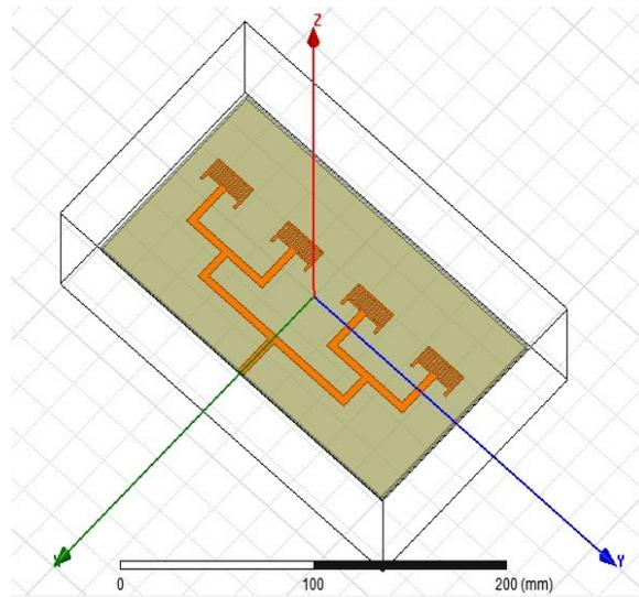
Figure5. Design of 4x1 Slotted microstrip patch antenna
