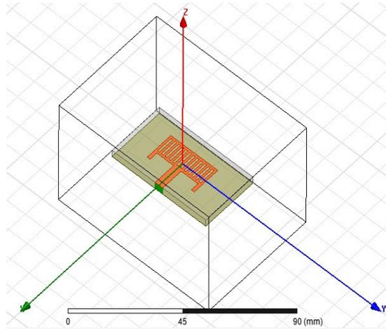
Figure1B. Design of slotted microstrip patch antenna
