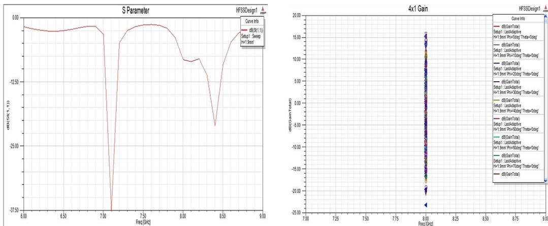
Figure6. Return Loss plot for 4x1 array
