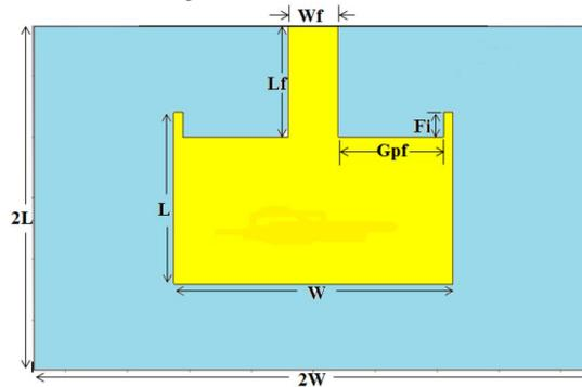
Figure1A. Schematic of Slotted microstrip patch antenna
