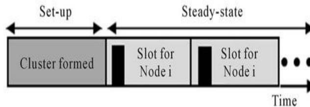
Fig.2. Timeline Showing LEACH Protocol Operation
