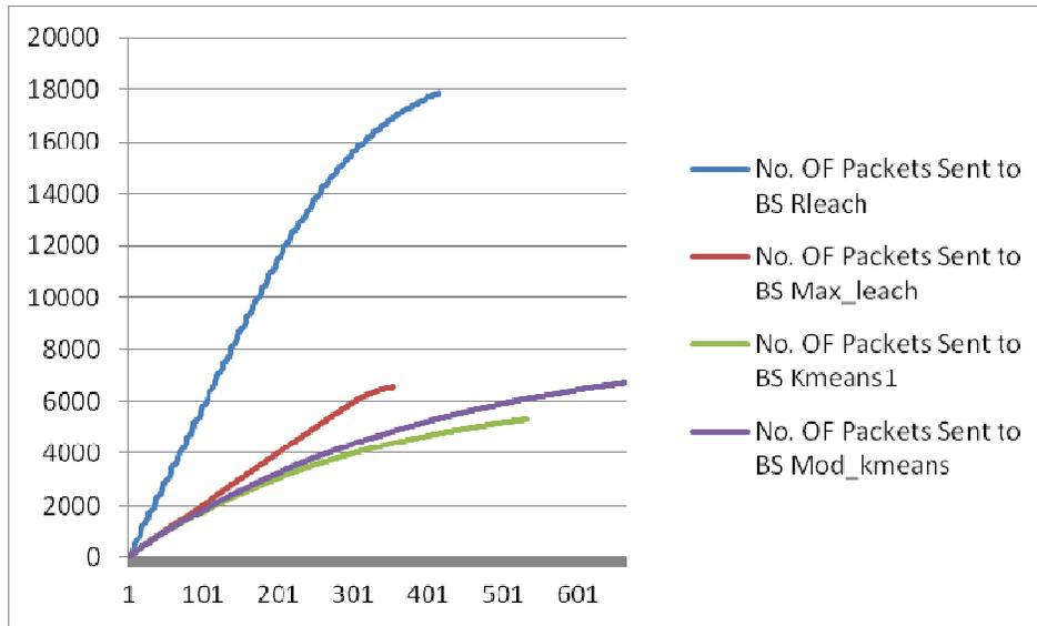
**Fig 8: Comparison of four algorithms for no of packets sent to BS Vs No. of Rounds**
