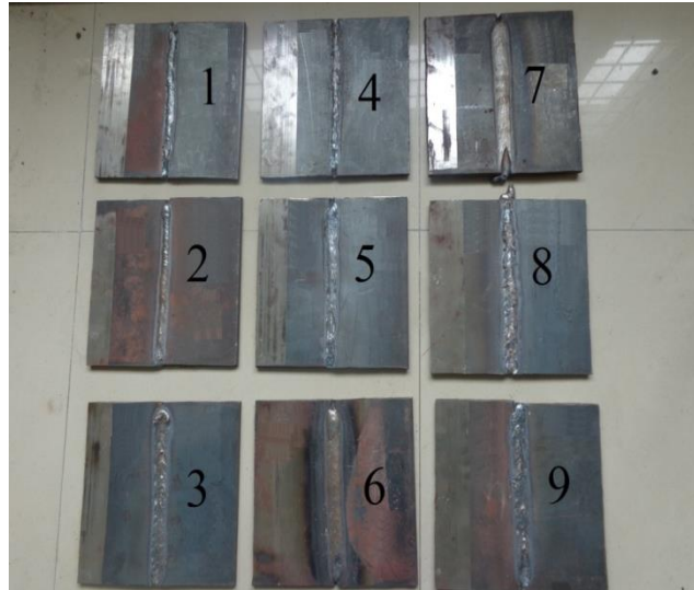
Fig. 2 Plates after welding.
