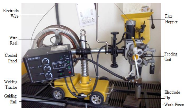
Fig. 1 SAW set-up used for experimentation
