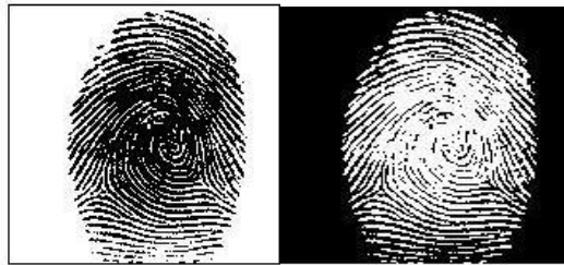
Figure 9: Segmented fingerprint of good quality image taken from DB1 and Gabor filter image of good quality
