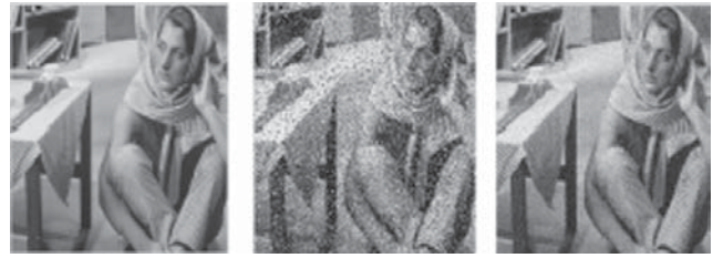
Figure 5: The Barbara Gray Image Corrupted with a High Level of Nixed Noise ( p = 60\% ) and the Results of Applying Two Stage Trilateral Filter
