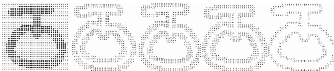
Figure 1: (a) Binary Image 34x34 Pixels Size. Its GM Computed using (b) Frei-Chen Operator, (c) Prewitt Operator, (d) Sobel Operator and (e) Robert Operator
