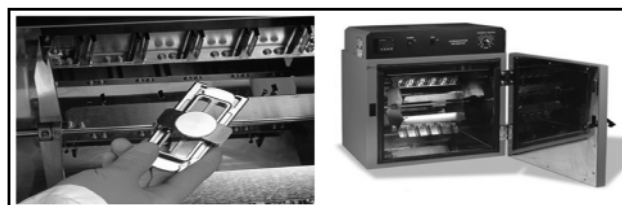
Fig.5: Hybridization Chamber (Arrow Indicates the Gasket which Holds the Micro Array Slide and Placed in the Hybridization Chamber)
