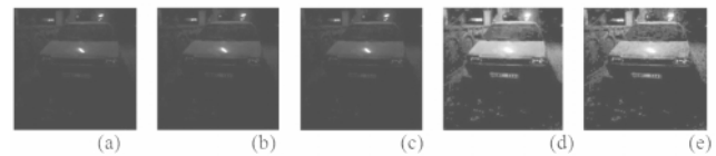
Fig.8 (a) Original Image (b) SSR Image (c) MSR Image (d) MSRCR Image (e) Homomorphic Filtering
