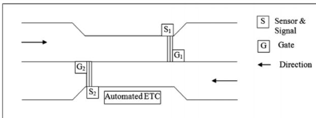
Figure 1: Showing the Arrangement of Automated ETC
