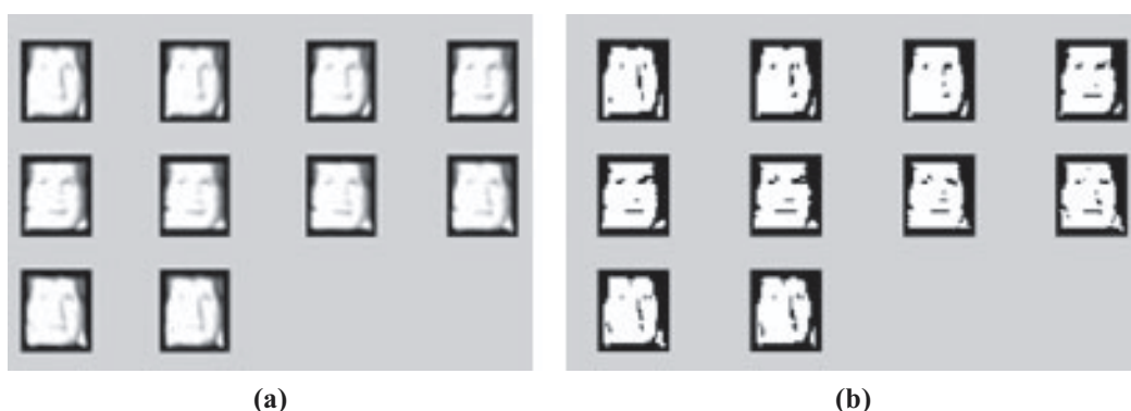
Figure 3 (a) Convolved Face Image at Different Orientations and Frequency 0.20 (b) Threshold Face Image After Gabor Features are Extracted
